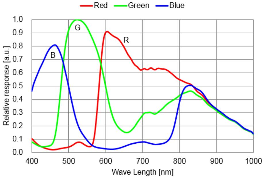
Figure 4-3 VEN-505-36U3C-(M01/M05/M06) sensor spectral response
