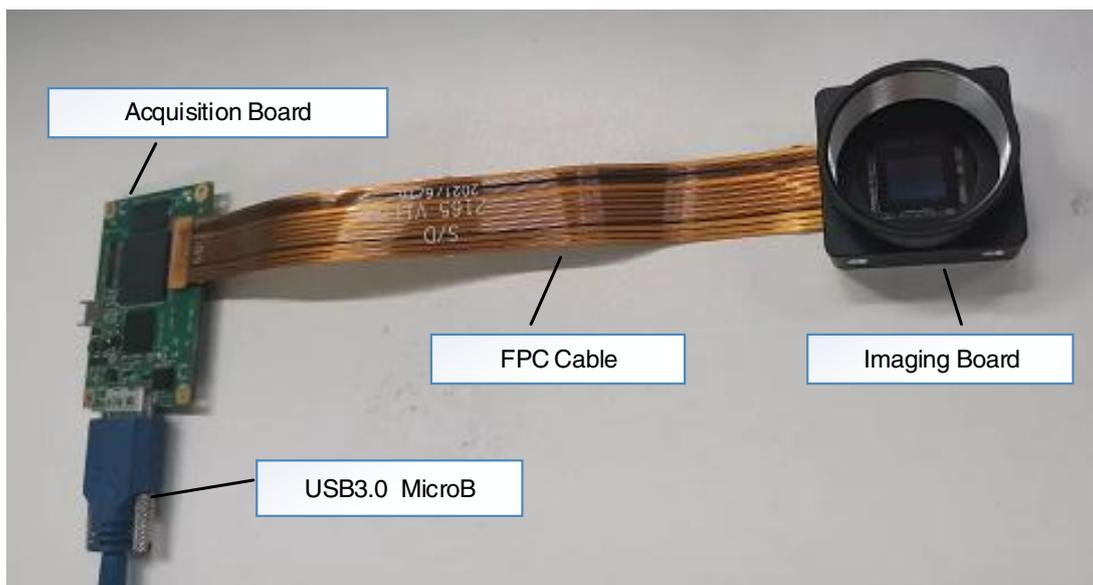
Figure 3-3 Split USB3.0 camera composition diagram (C-Mount)
