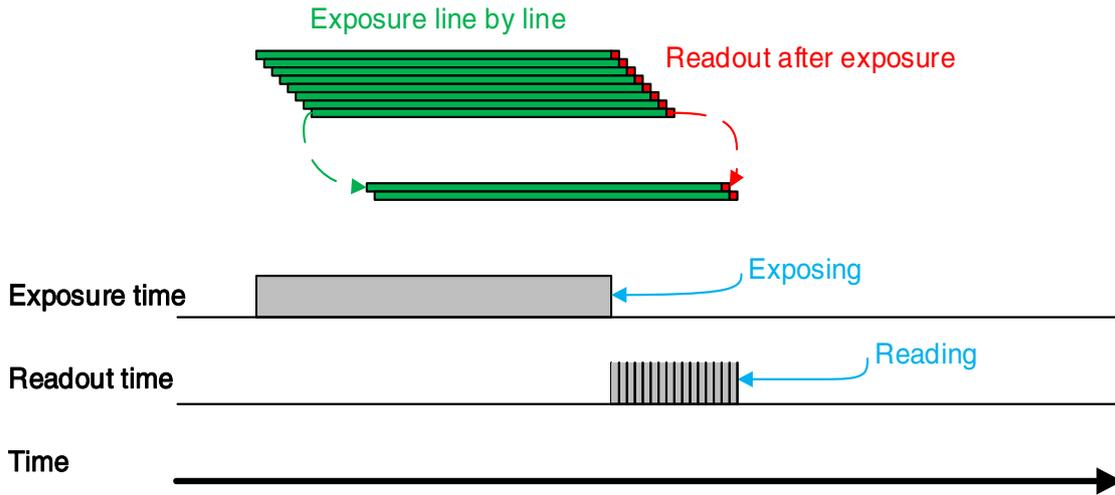
Figure 8-25 Electronic rolling shutter
