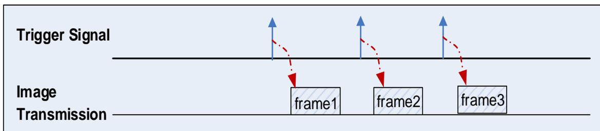
Figure 8-14 FrameStart trigger
