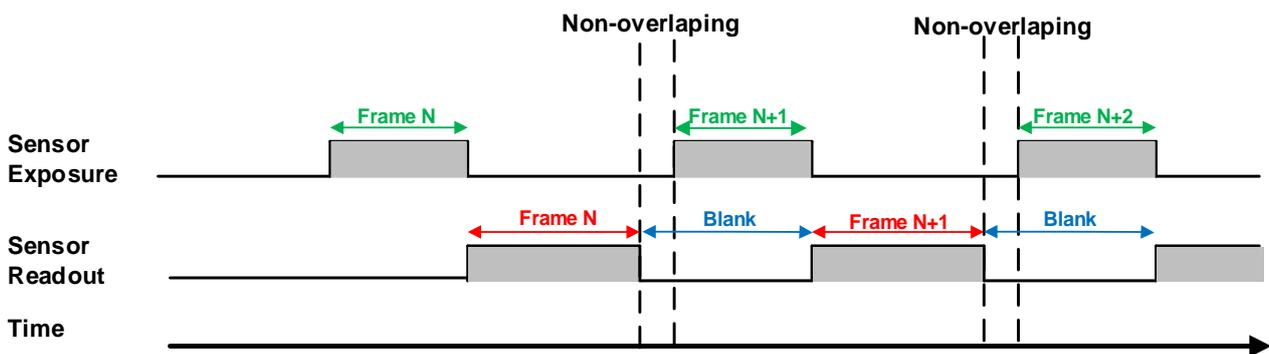
Figure 8-27 The exposure sequence diagram in non-overlapping exposure mode
