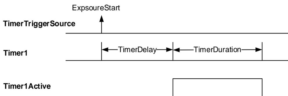
Figure 8-59 Timer1Active schematic diagram
