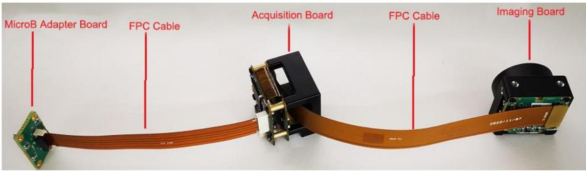
Figure 3-17 Split vertical FPC camera's hardware composition
