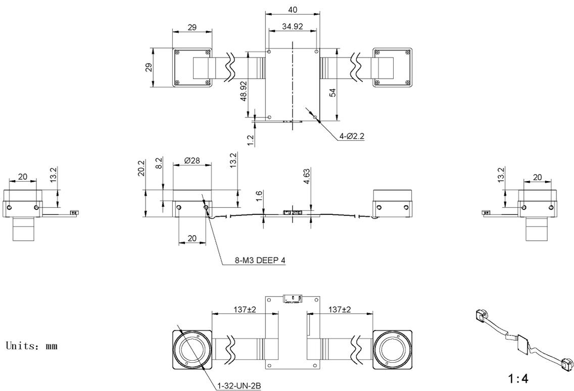
Figure 5-11 Split USB3.0 binocular camera mechanical dimensions (C-Mount)
