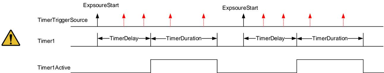
Figure 8-60 The relationship of Timer1Active and ExposureStart signal
