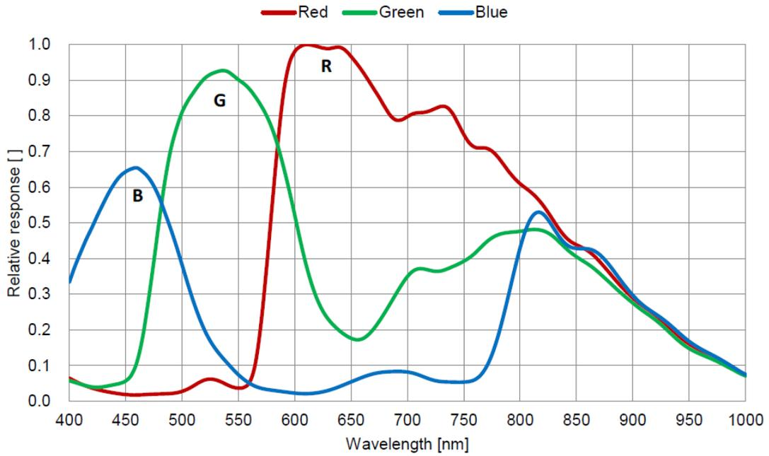
Figure 4-7 VEN-302-56U3C-S sensor spectral response
