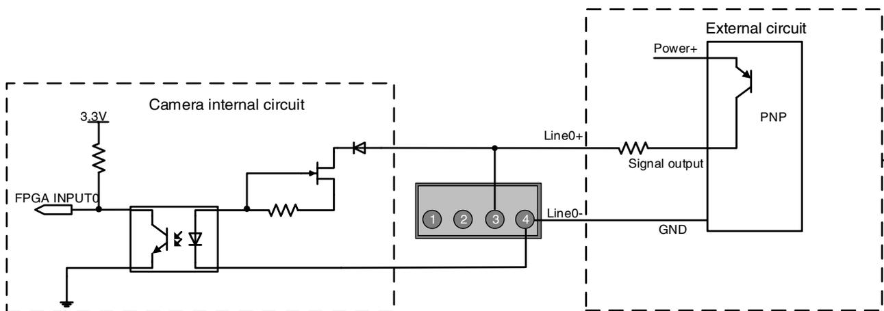
Figure 7-4 PNP photosensor connected to opto-isolated input circuit
