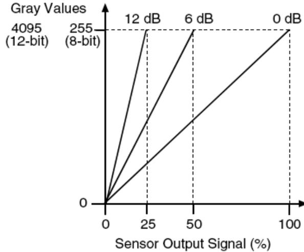
Figure 8-31 The camera's response curve
