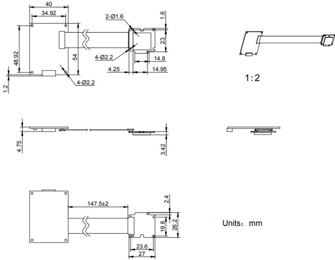
Figure 5-10 Split USB3.0 camera mechanical dimensions (No-Mount)
