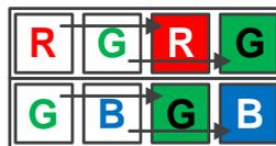
Figure 8-41 Horizontal color Binning by 2
