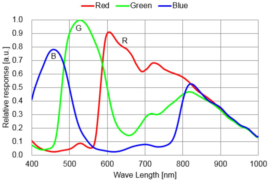
Figure 4-5 VEN-830-22U3C-(M01/M05/M06) sensor spectral response
