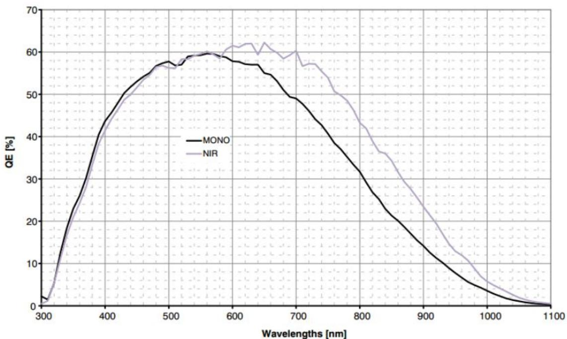
Figure 4-10 VEN-134-90U3M-D NIR sensor spectral response
