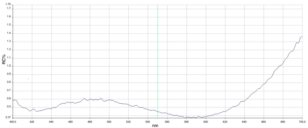
Figure 6-2 Transparent glass reflectance curve for VENUS USB3 Vision series mono camera
