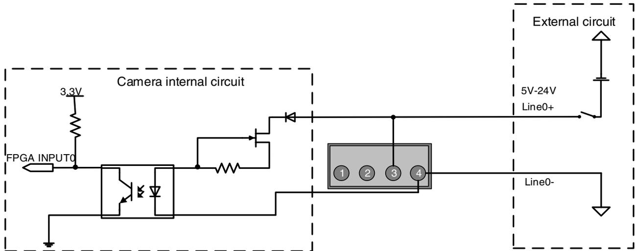
Figure 7-2 Opto-isolated input circuit
