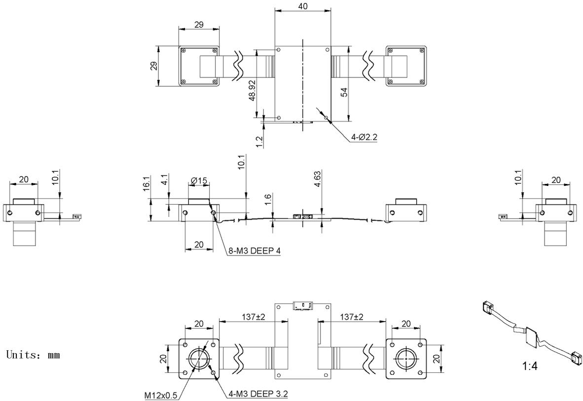
Figure 5-13 Split USB3.0 binocular camera mechanical dimensions (S-Mount)
