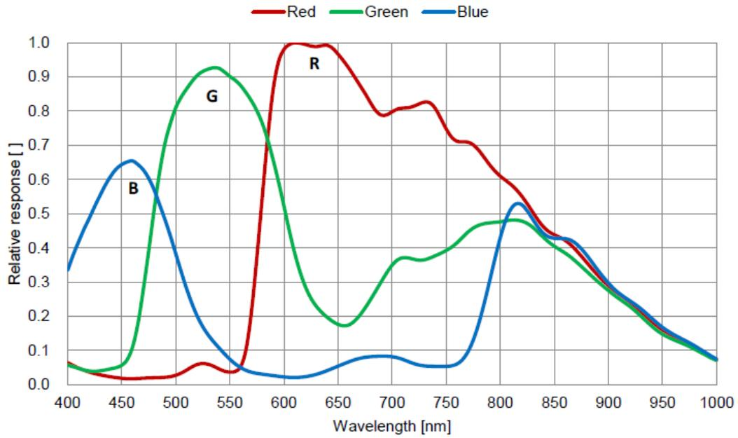
Figure 4-19 VE2S-301-125U3C-S (J150) sensor spectral response
