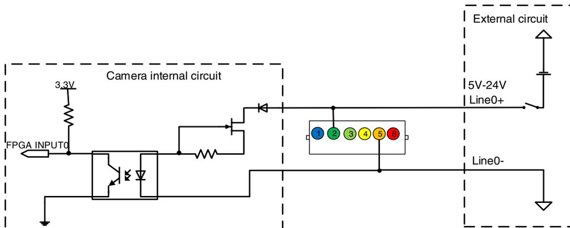
Figure 7-29 Opto-isolated input circuit
