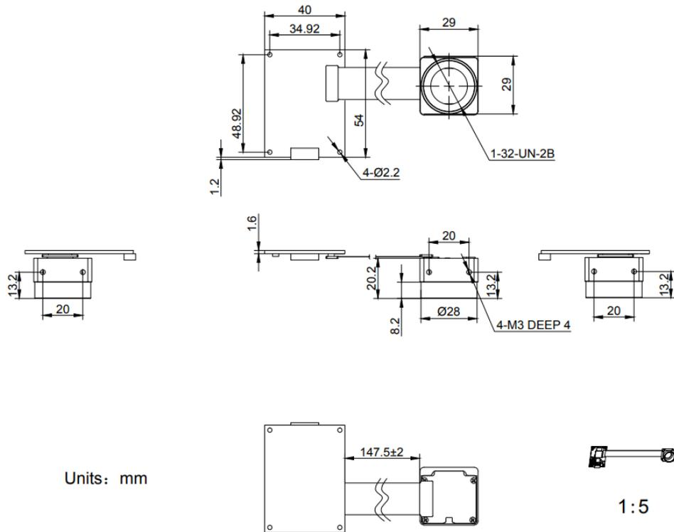
Figure 5-9 Split USB3.0 camera mechanical dimensions (C-Mount)
