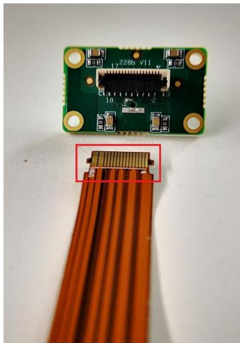
Figure 3-16 FPC cable connect to the Micro-B adapter board
