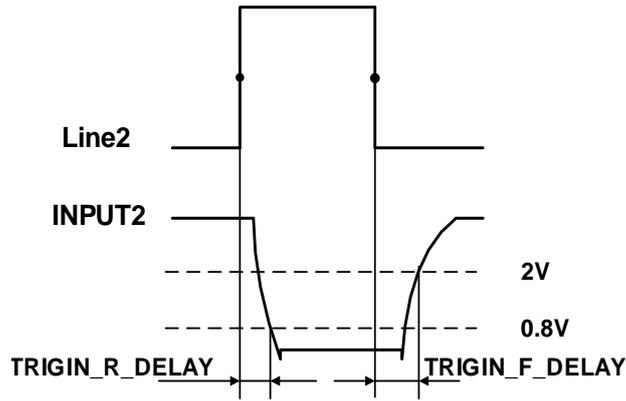
Figure 7-10 Parameter of Line2 input circuit
