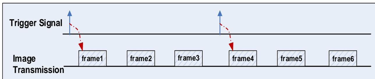
Figure 8-15 FrameBurstStart trigger
