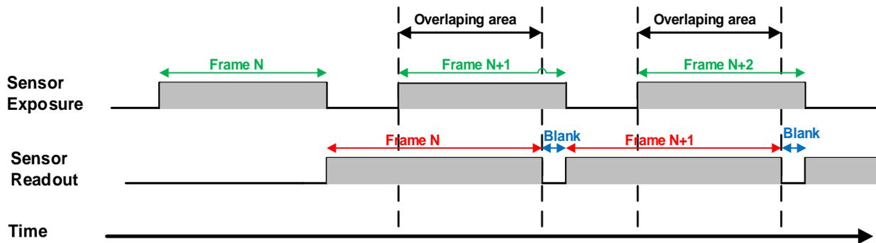
Figure 8-29 The exposure sequence diagram in overlapping exposure mode
