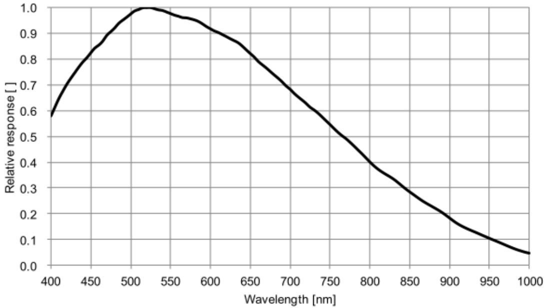
Figure 4-14 VEN-230-168U3M-FPC sensor spectral response
