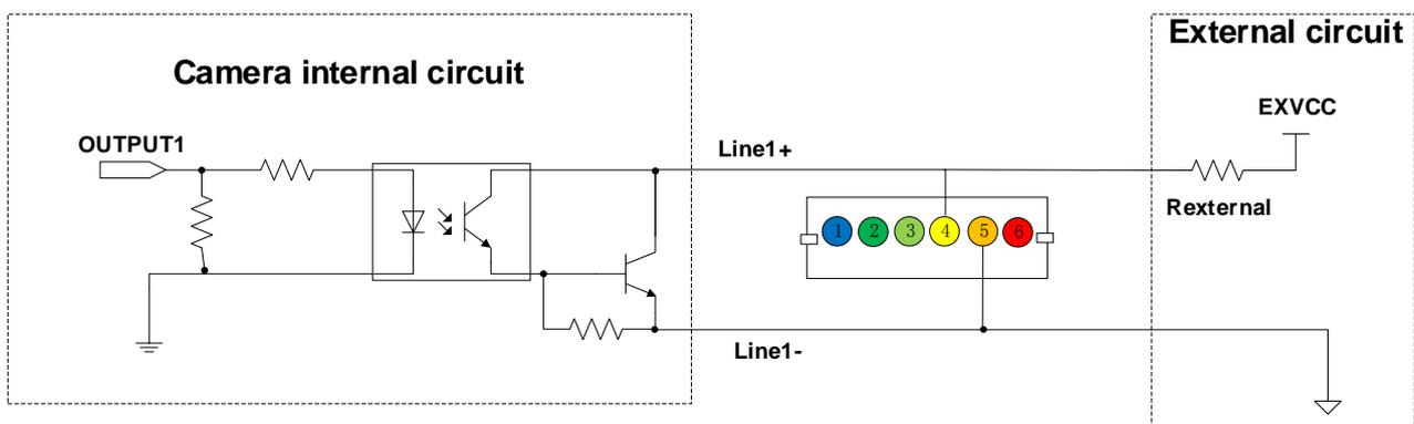
Figure 7-33 Opto-isolated output circuit
