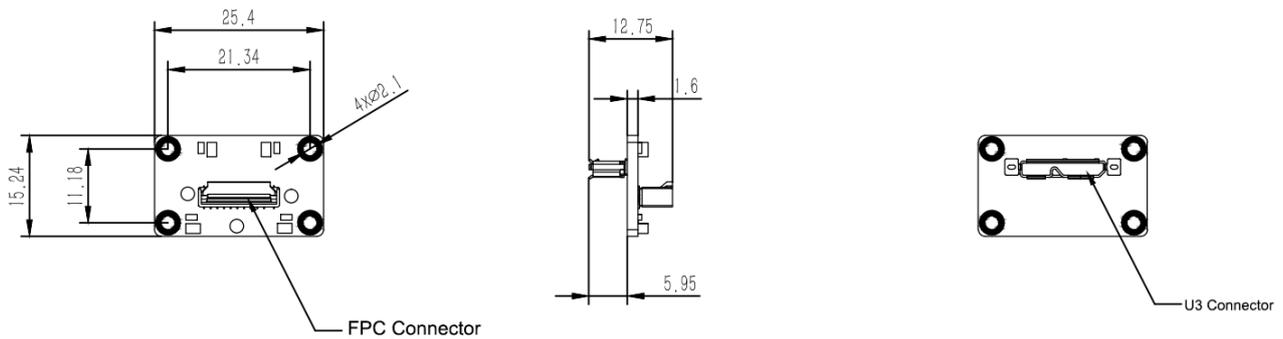
Figure 5-16 Micro-B adapter board mechanical dimensions
