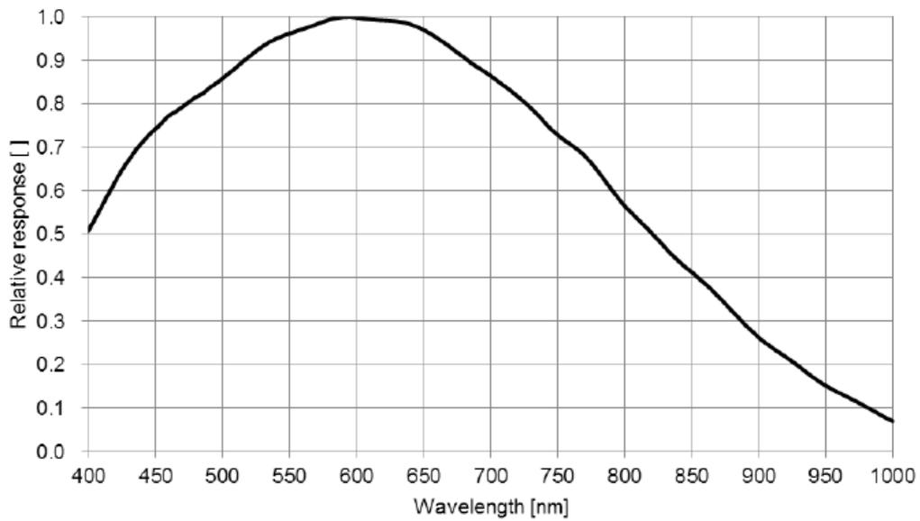
Figure 4-20 VE2S-301-125U3M-S (J150) sensor spectral response
