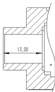
Figure 5-20 S-mount optical interface of VENUS all-in-one FPC camera
