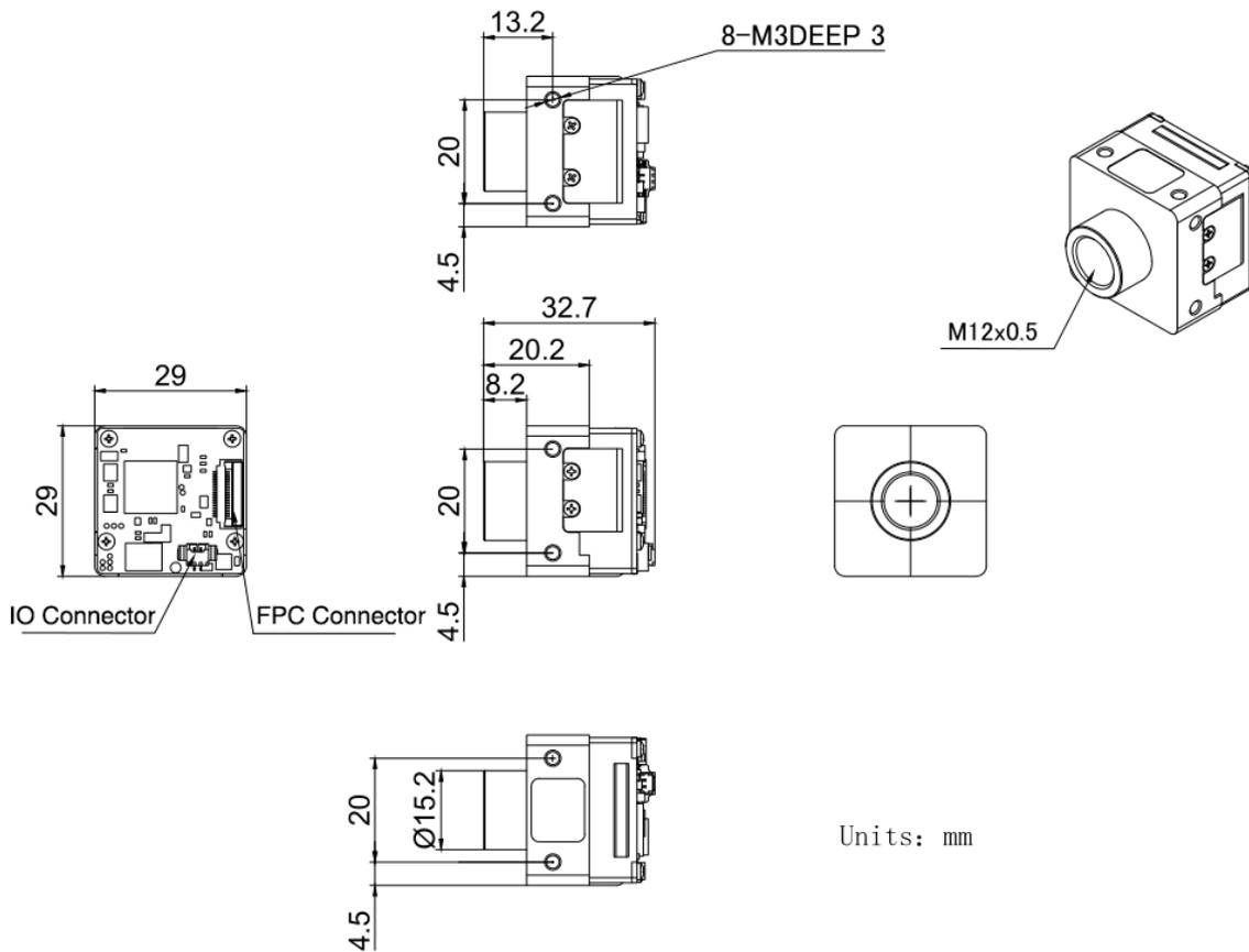
Figure 5-7 All-in-one horizontal FPC camera mechanical dimensions (S-Mount)
