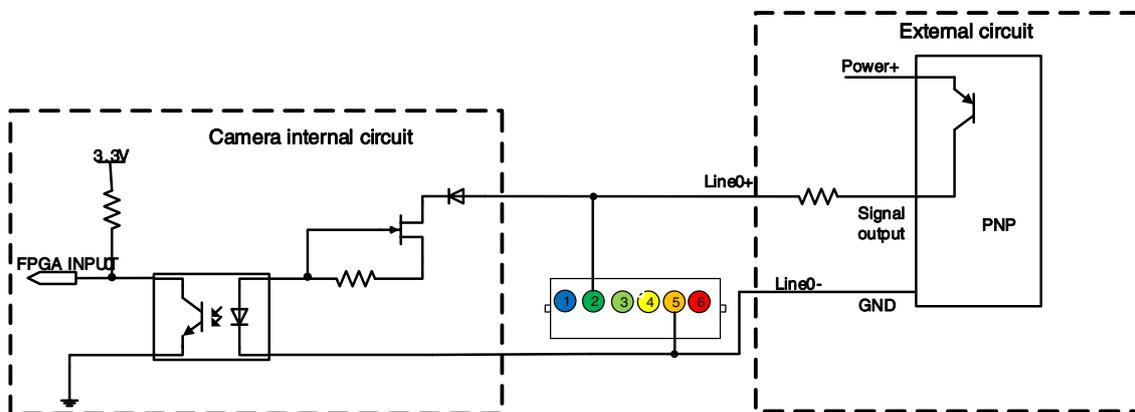
Figure 7-31 PNP photosensor connected to opto-isolated input circuit
