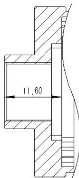
Figure 5-19 S-mount optical interface of VENUS USB3 Vision camera (except FPC camera)
