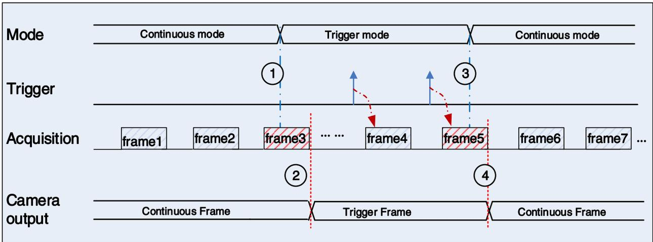
Figure 8-17 Switch trigger mode during frame reading out
