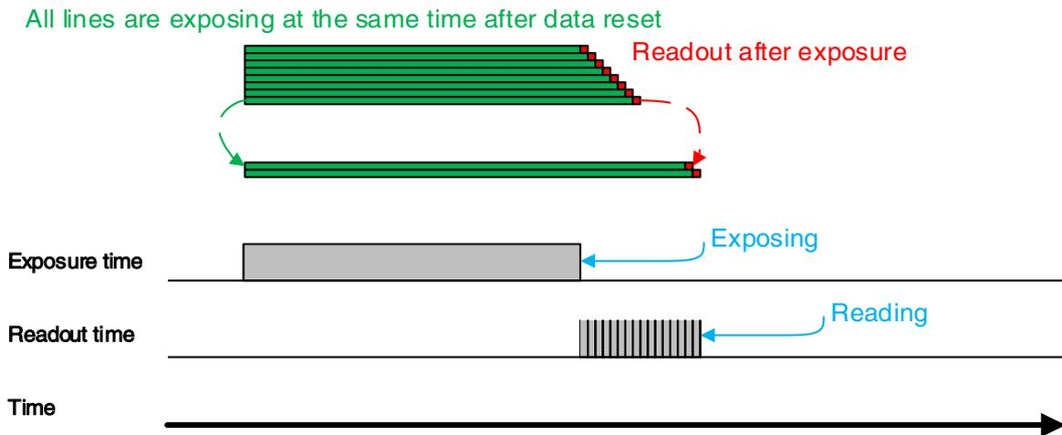
Figure 8-26 Global reset rolling shutter
