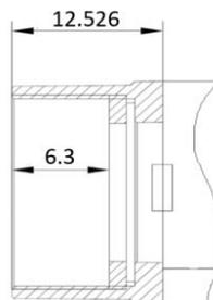
Figure 5-18 CS-mount optical interface of VENUS USB3 Vision camera
