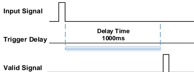
Figure 8-2 Trigger delay schematic diagram
