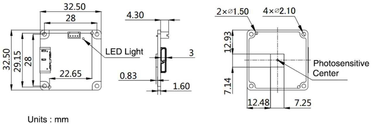
Figure 5-4 VEN-505-36U3M/C-M06 mechanical dimensions
