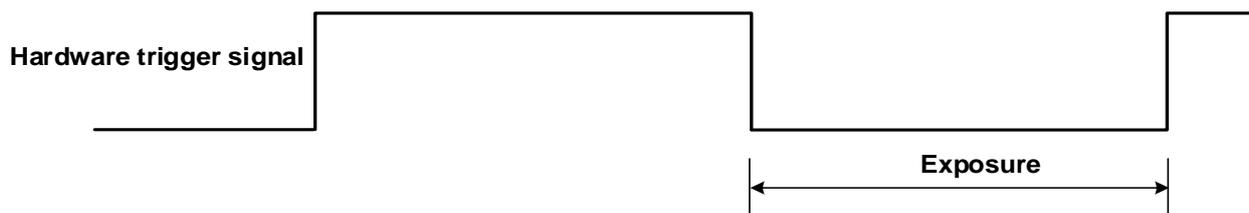
Figure 8-23 The sequence diagram in falling edge trigger of TriggerWidth exposure mode
