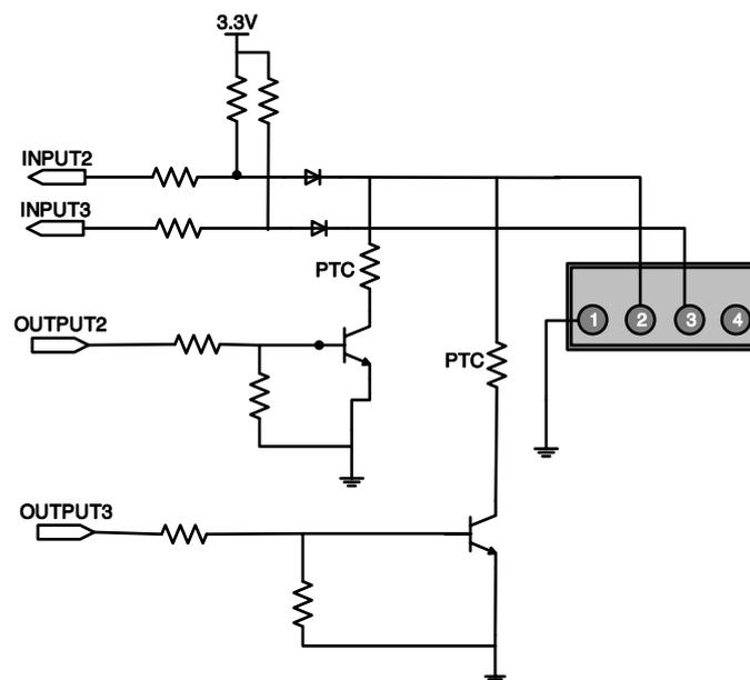
Figure 7-14 Line2/3 (bidirectional) circuit
