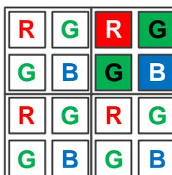
Figure 8-43 Horizontal and vertical color Binning by 2x2
