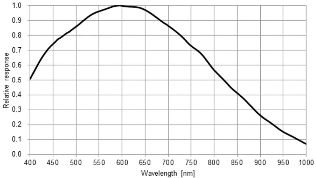
Figure 4-8 VEN-302-56U3M-S sensor spectral response
