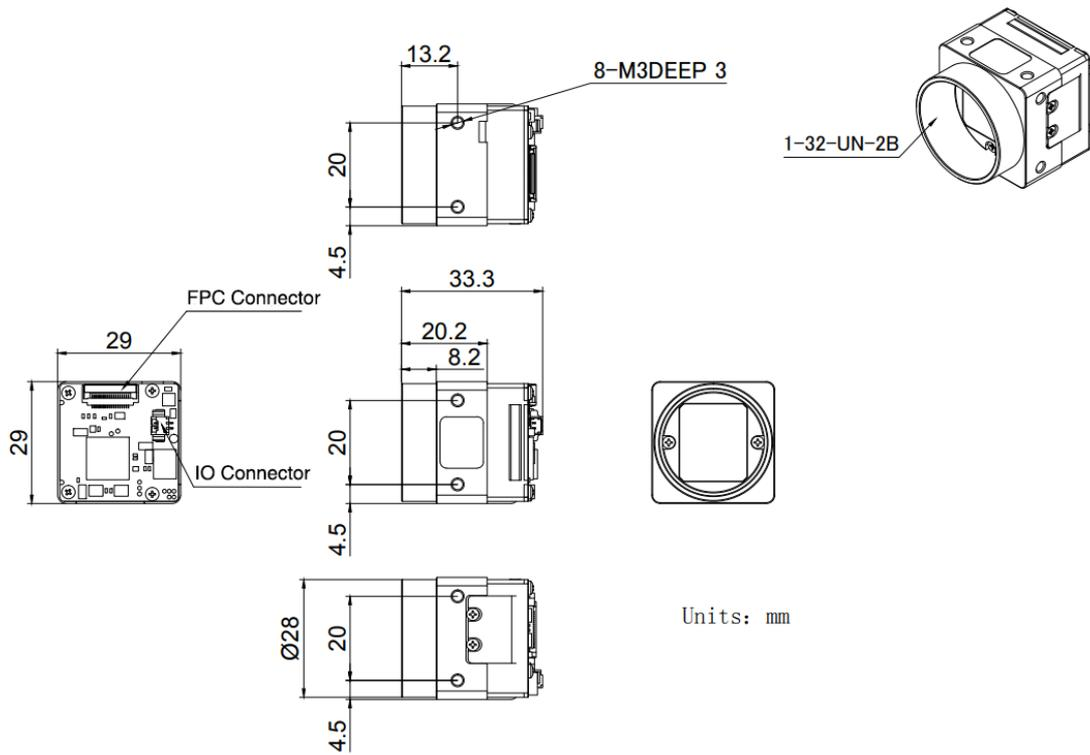
Figure 5-6 All-in-one horizontal FPC camera mechanical dimensions (C-Mount)
