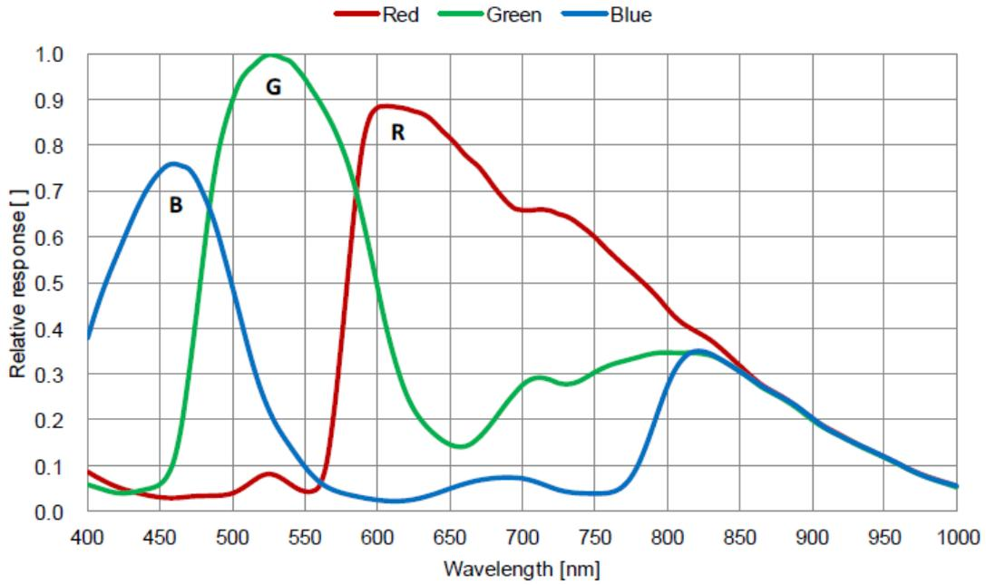
Figure 4-13 VEN-230-168U3C-FPC sensor spectral response
