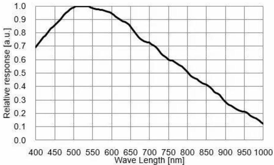
Figure 4-4 VEN-505-36U3M-(M01/M05/M06) sensor spectral response
