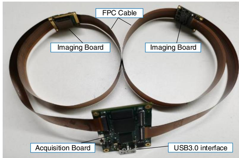
Figure 3-4 Split binocular USB3.0 interface camera composition diagram (without C-Mount)
