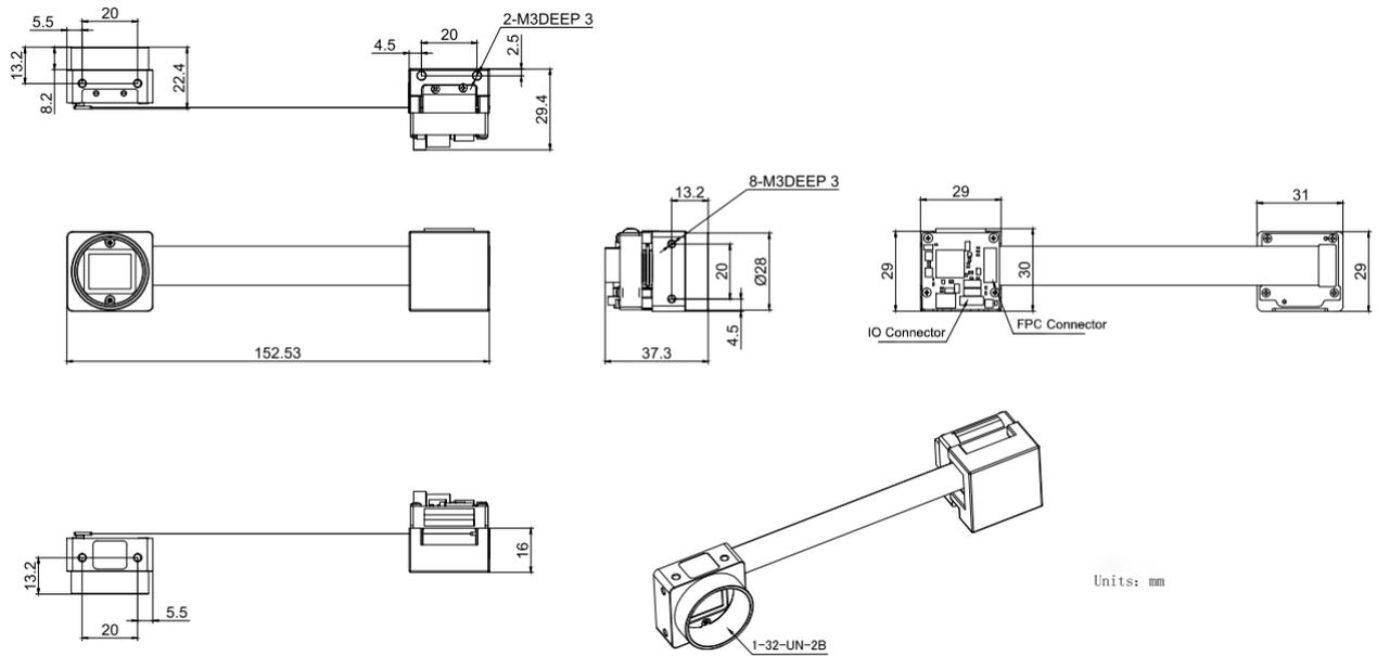
Figure 5-15 Split vertical FPC camera mechanical dimensions
