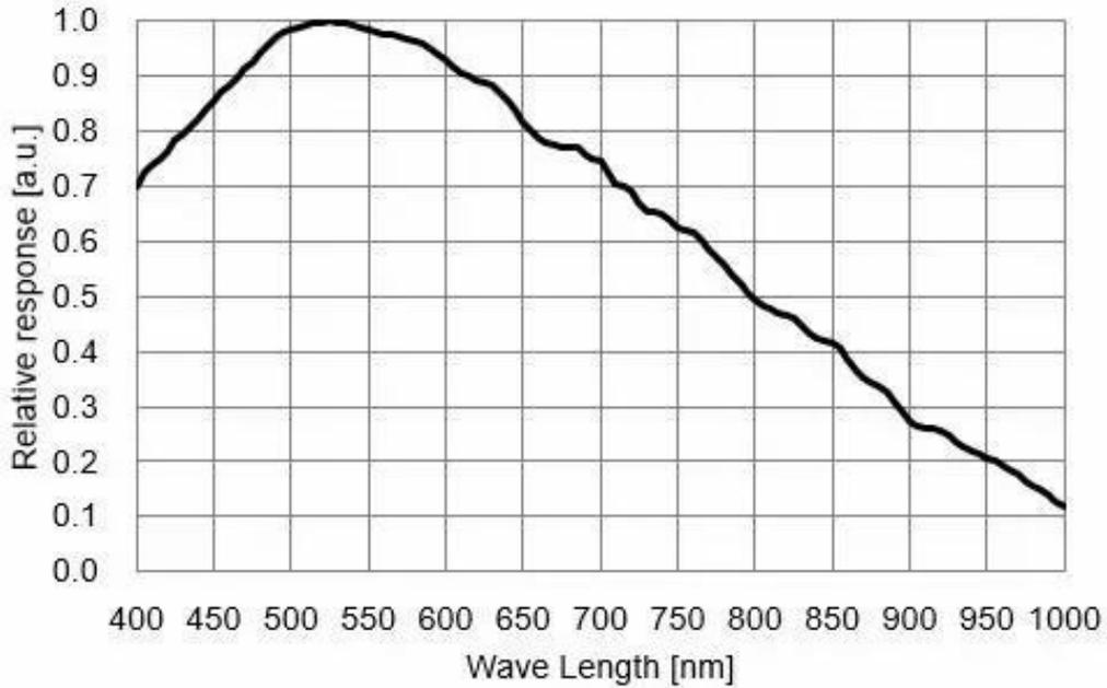
Figure 4-6 VEN-830-22U3M-(M01/M05/M06) sensor spectral response
