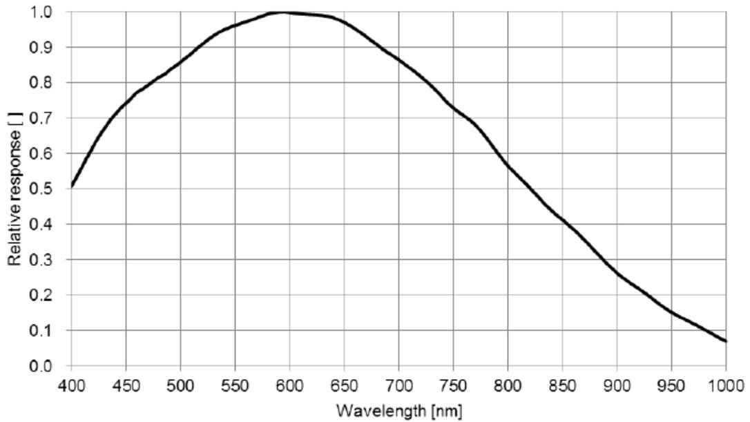
Figure 4-16 VEN-301-125U3M-FPC sensor spectral response
