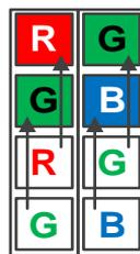
Figure 8-42 Vertical color Binning by 2
