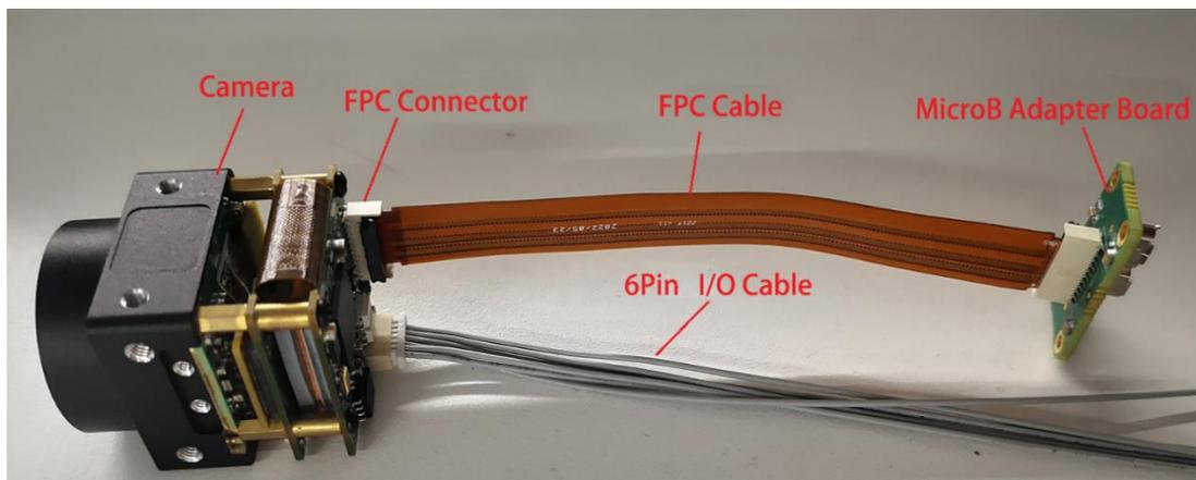
Figure 3-14 All-in-one vertical FPC camera's hardware composition
