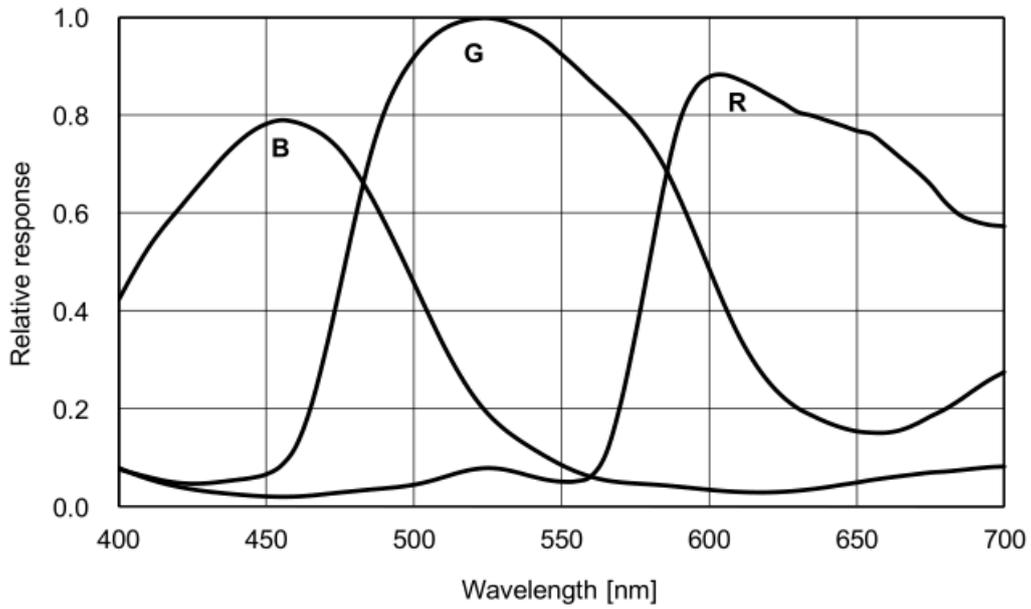
Figure 4-17VEN-1220-32U3C-FPC sensor spectral response
