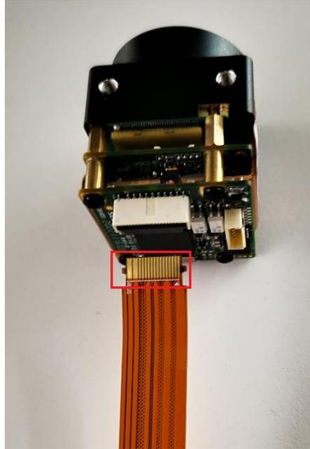
Figure 3-15 FPC cable connect to the camera
