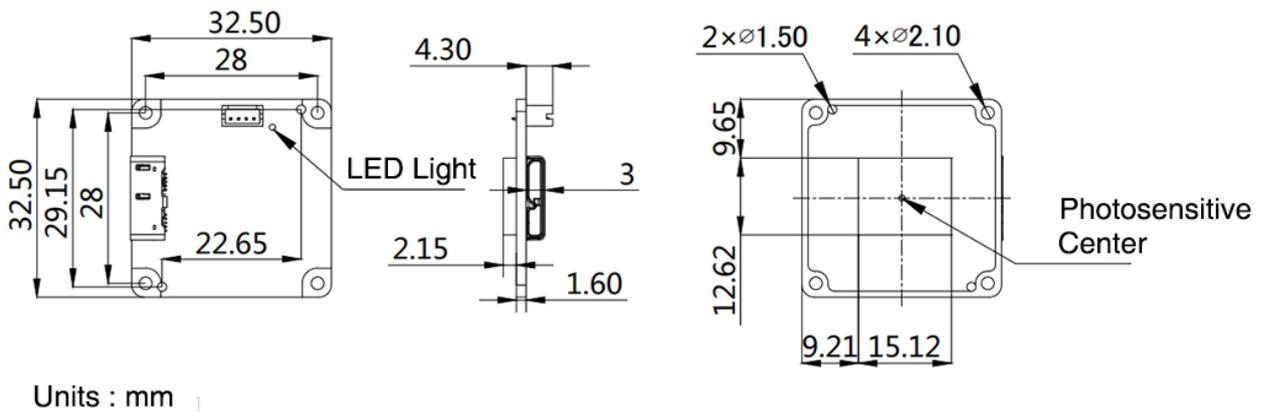
Figure 5-5 VEN-830-22U3M/C-M06 mechanical dimensions
