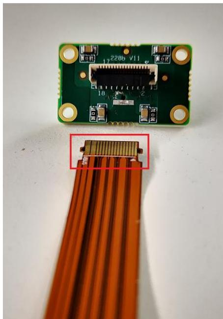
Figure 3-21 FPC cable connect to the Micro-B adapter board
