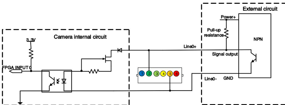
Figure 7-30 NPN photosensor connected to opto-isolated input circuit
