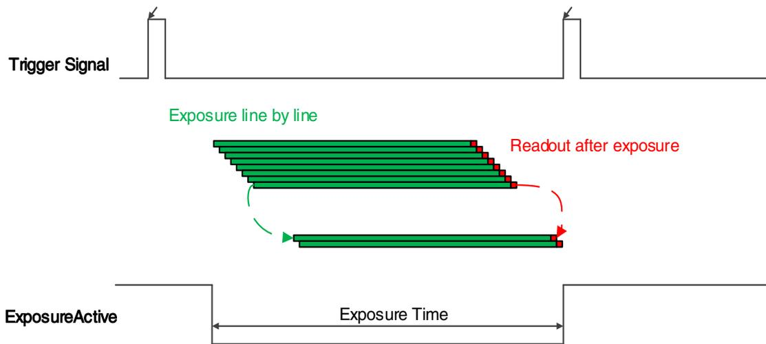
Figure 8-6 Electronic rolling shutter "ExposureActive" signal schematic diagram
