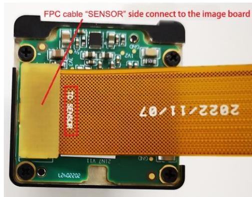
Figure 3-18 FPC cable connect to the image board
