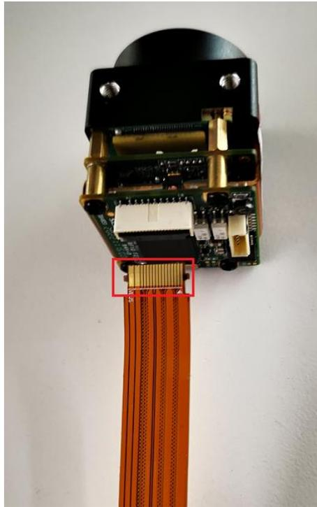
Figure 3-20 FPC cable connect to the FPC holder
