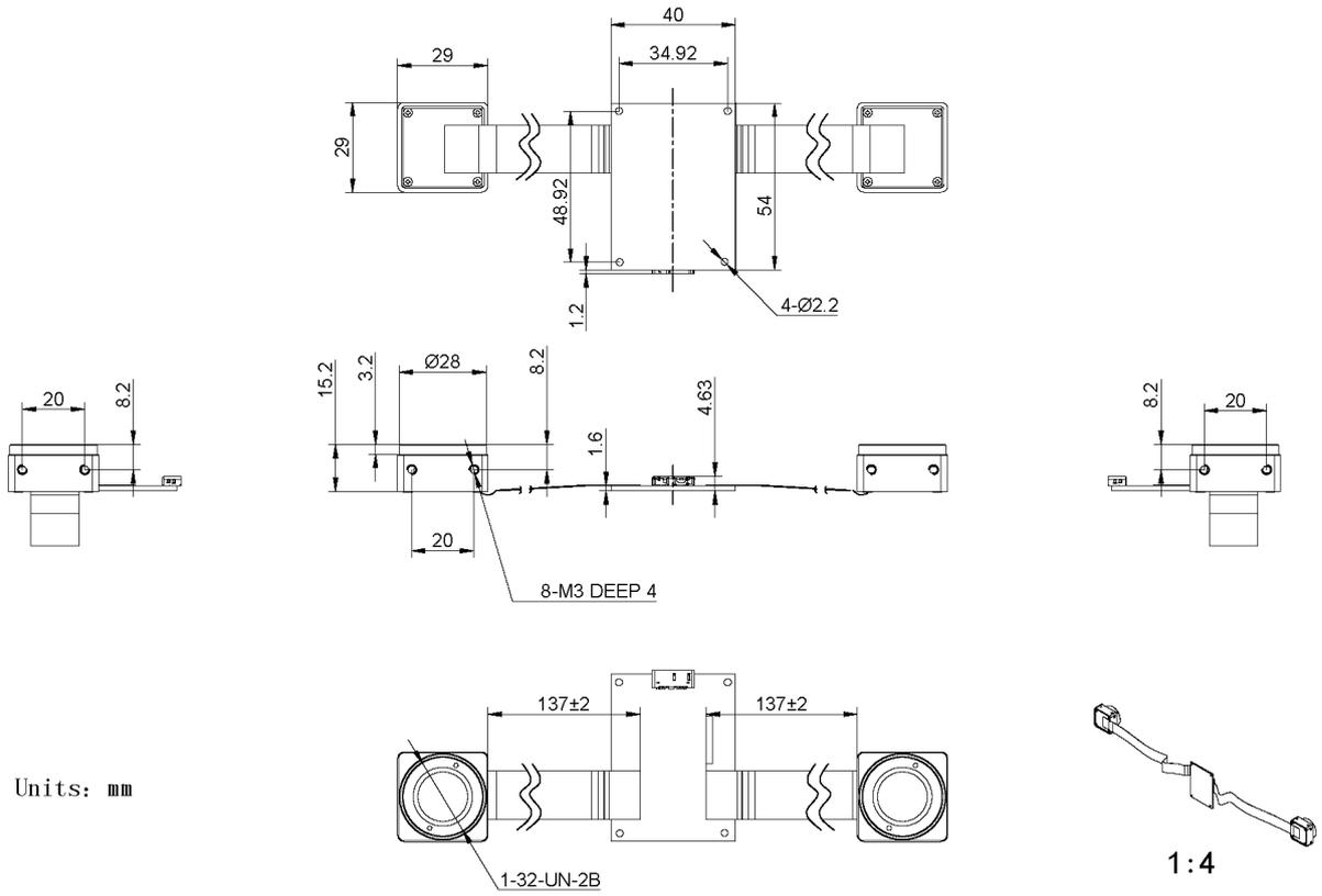
Figure 5-12 Split USB3.0 binocular camera mechanical dimensions (CS-Mount)
