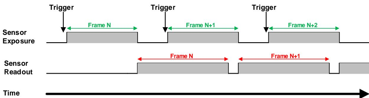
Figure 8-30 The trigger acquisition exposure sequence diagram in overlapping exposure mode
