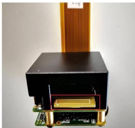
Figure 3-19 FPC cable connect to the acquisition board
