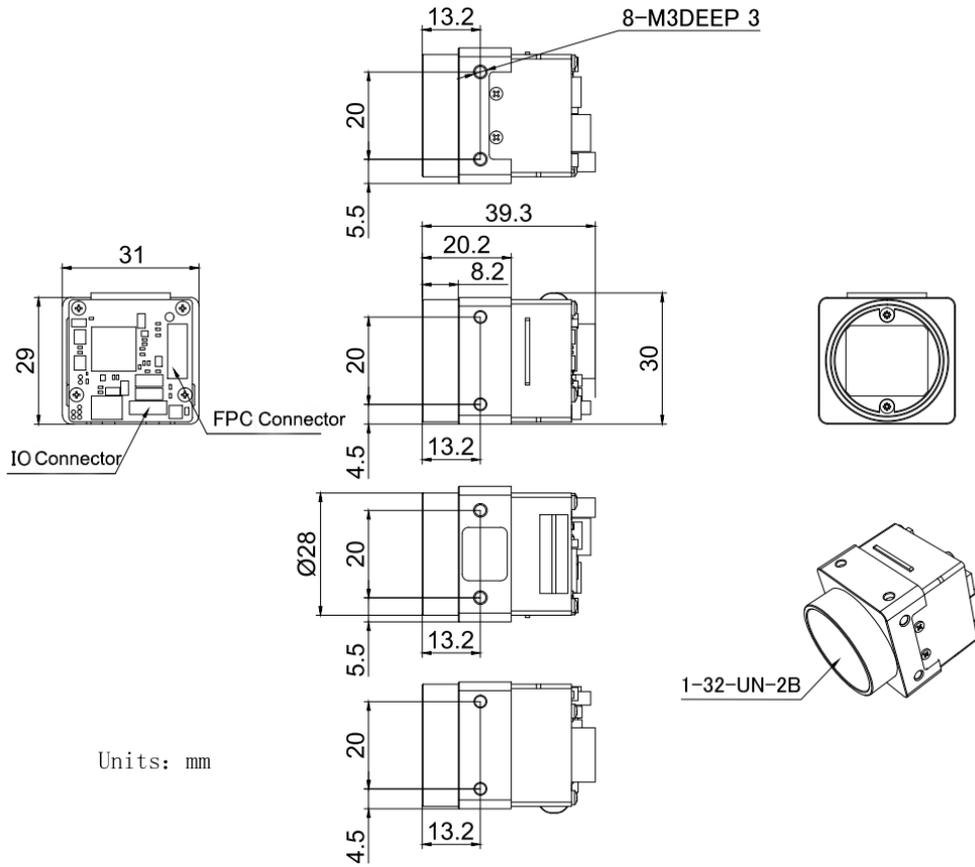
Figure 5-8 All-in-one vertical FPC camera mechanical dimensions
