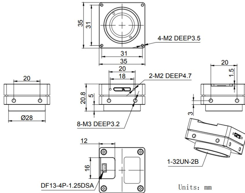
Figure 5-1 All-in-one USB3.0 camera mechanical dimensions (CS-Mount)
