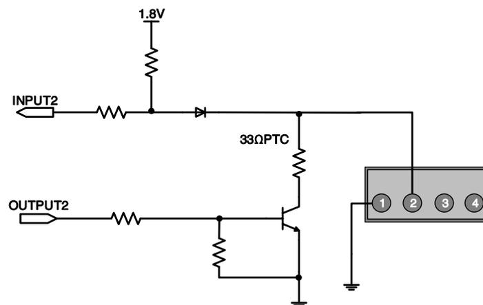
Figure 7-6 Line2 (bidirectional) circuit
