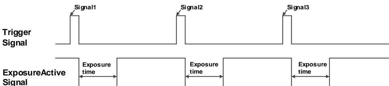
Figure 8-5 Global shutter "ExposureActive" signal schematic diagram
