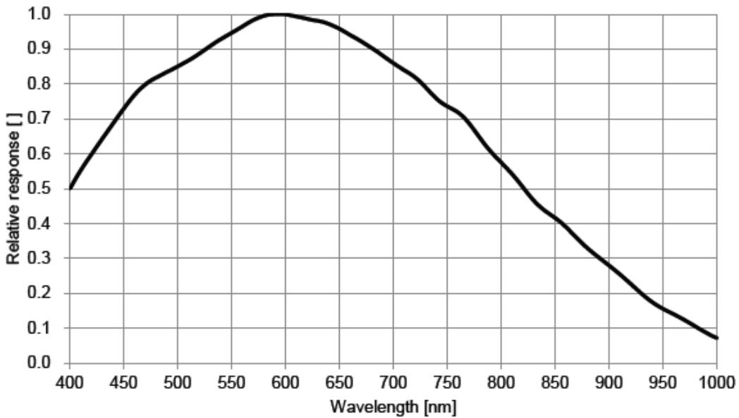
Figure 4-12 VEN-160-227U3M-FPC-(M00/M05) sensor spectral response
