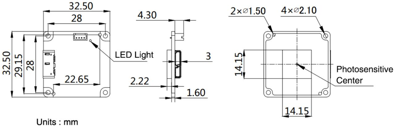
Figure 5-3 VEN-161-61U3M/C-M06 mechanical dimensions
