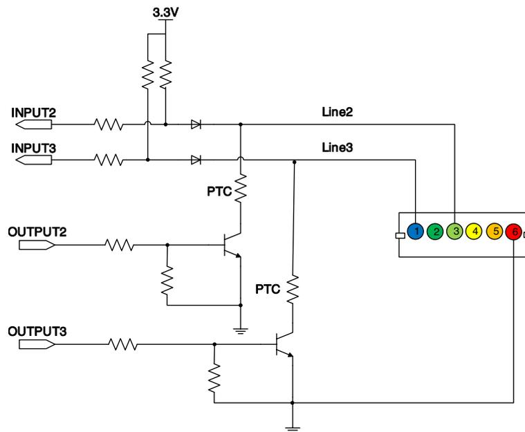
Figure 7-35 Line2/3 (bidirectional) circuit
