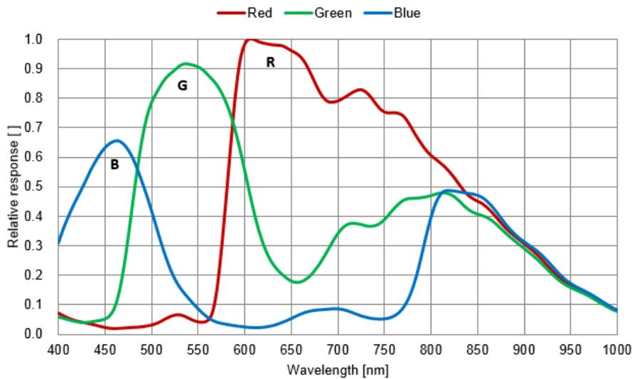
Figure 4-1 VEN-161-61U3C-(M01/M05/M06) sensor spectral response
