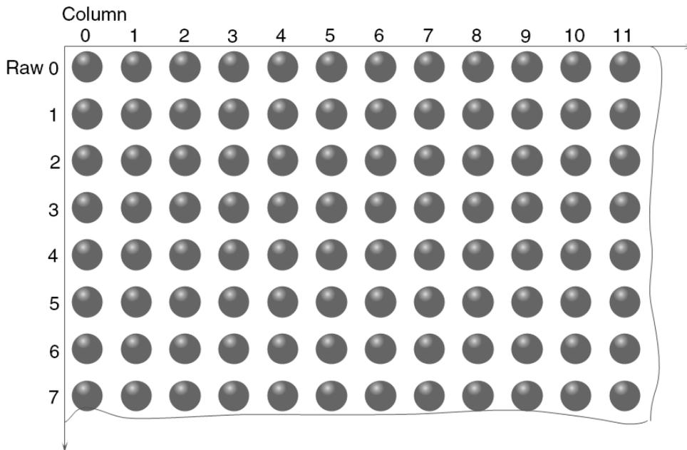
Figure 8-32 Mono8 pixel format
