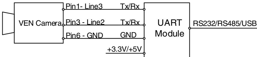
Figure 8-70 The wiring diagram of the camera and external serial port device
