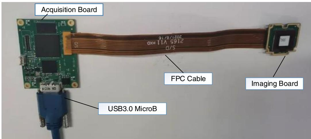
Figure 3-2 Split USB3.0 camera composition diagram (without C-Mount)
