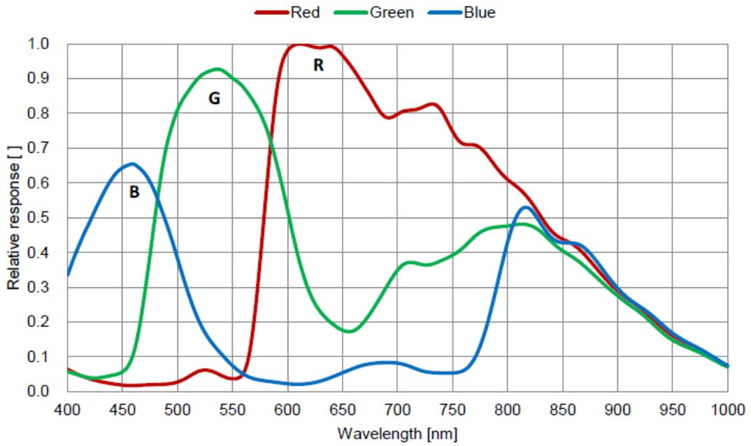
Figure 4-15 VEN-301-125U3C-FPC sensor spectral response
