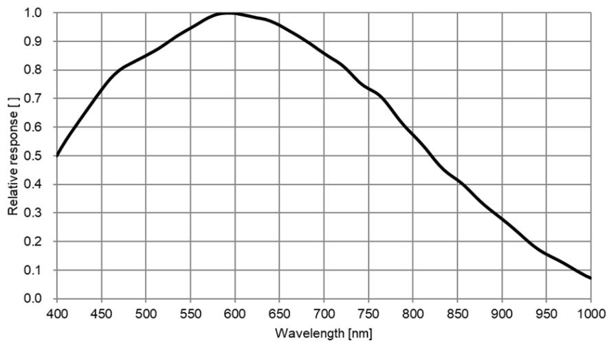
Figure 4-2 VEN-161-61U3M-(M01/M05/M06) sensor spectral response
