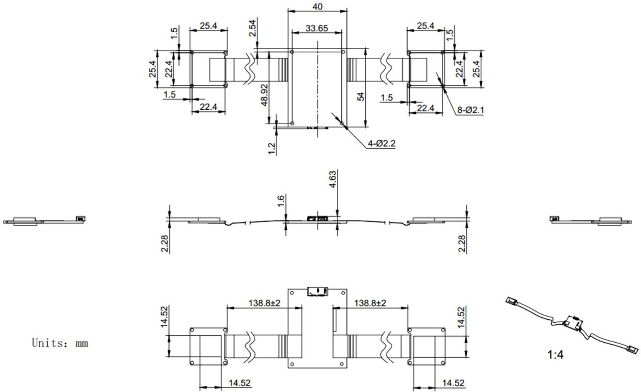
Figure 5-14 Split USB3.0 binocular camera mechanical dimensions (No-Mount)
