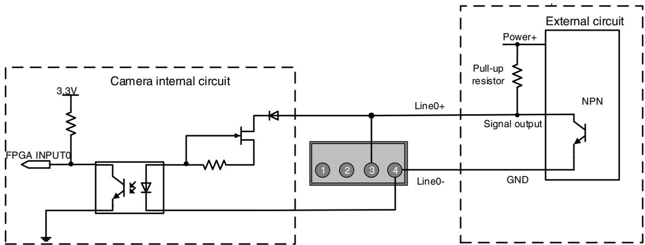
Figure 7-3 NPN photosensor connected to opto-isolated input circuit
