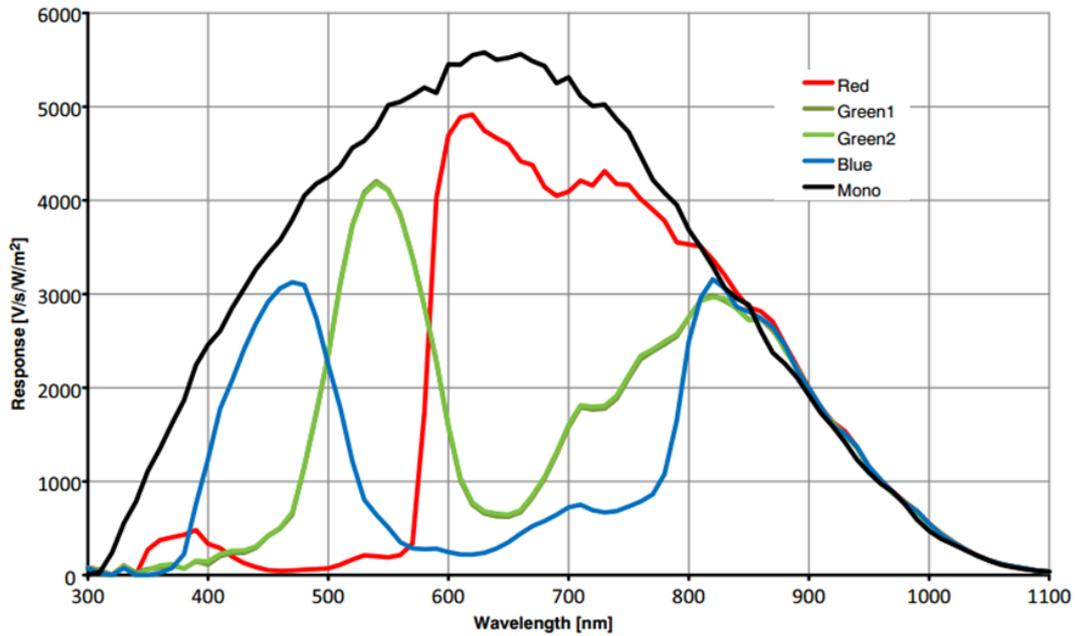
Figure 4-9 VEN-134-90U3M/C-D sensor spectral response
