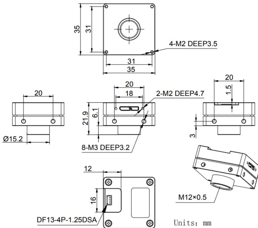
Figure 5-2 All-in-one USB3.0 camera mechanical dimensions (S-Mount)
