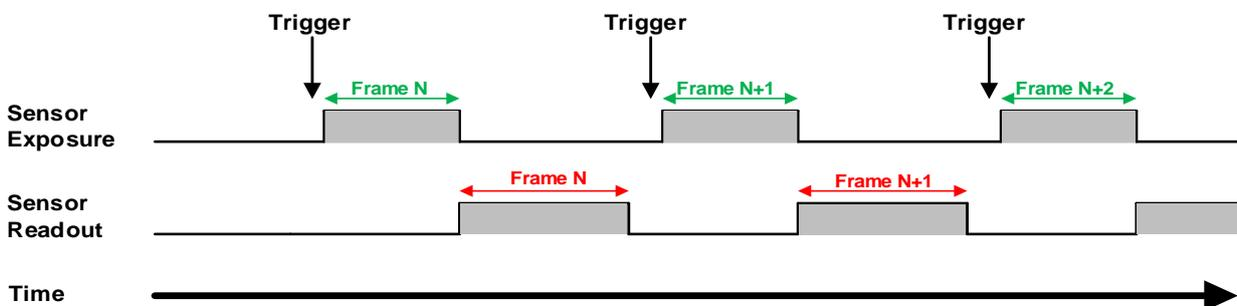
Figure 8-28 The trigger acquisition exposure sequence diagram in non-overlapping exposure mode
