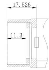
Figure 5-17 C-mount optical interface of VENUS USB3 Vision camera
