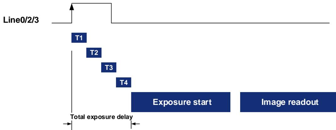
Figure 8-19 Exposure delay
