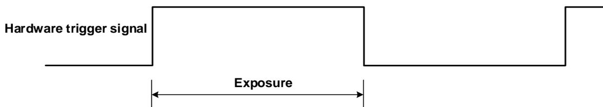
Figure 8-22 The sequence diagram in rising edge trigger of TriggerWidth exposure mode
