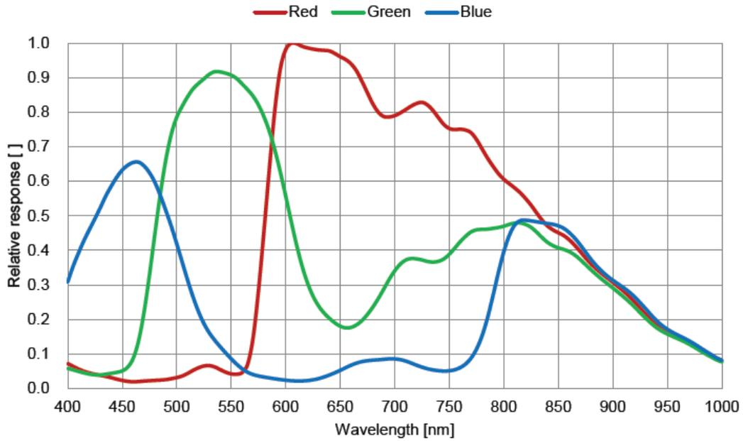
Figure 4-11 VEN-160-227U3C-FPC-(M00/M05) sensor spectral response
