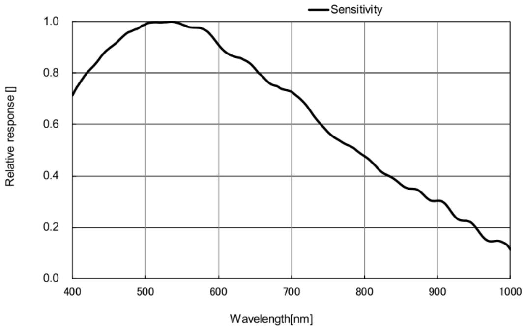
Figure 4-18 VEN-1220-32U3M-FPC sensor spectral response
